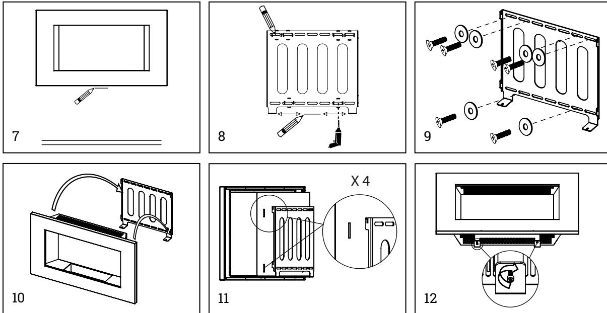
16. Lift the fireplace with the help of two people and hook it to the wall fixture. When the hooks are correctly placed, both the upper and lower hooks should lock into the fireplace (Figure 10-11). Check on both sides that both upper and lower hooks are correctly placed (Figure 11). **Important! If the hooks are not in the correct position, there is a higher risk that the fireplace will fall due to external force, so check this very carefully.**
