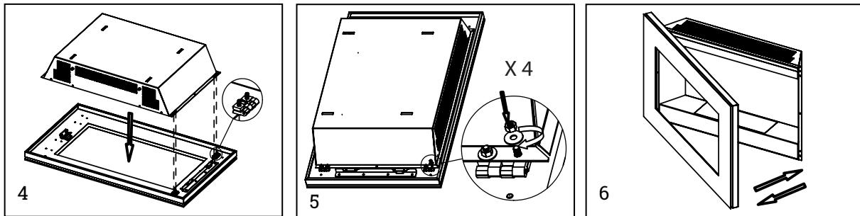
6. Mount screws according to Figure 2. Make sure the screws go in straight and without much resistance. Use an Allen wrench - tighten so that it is securely mounted. The front is now mounted - the fireplace is ready for installation on the wall. Go to point 12.
