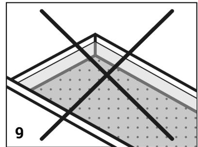
4. Be careful to avoid all spillage – any spill should be wiped off with a piece of paper. If overfilling occurs, use suitable utensils to remove excess fuel, so that the fuel comes level with the burner strainer.
