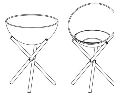
**Position the pivoted hemisphere on the tripod in such way that two standing legs are in front and one standing leg is behind the unit. Please make sure that the rear standing leg does not penetrate the hole of the hemisphere.**
