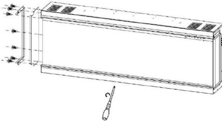
Fix back the fendig bars after the panels are removed. 3. Remove the screws from the fireplace as shown in the picture below.
