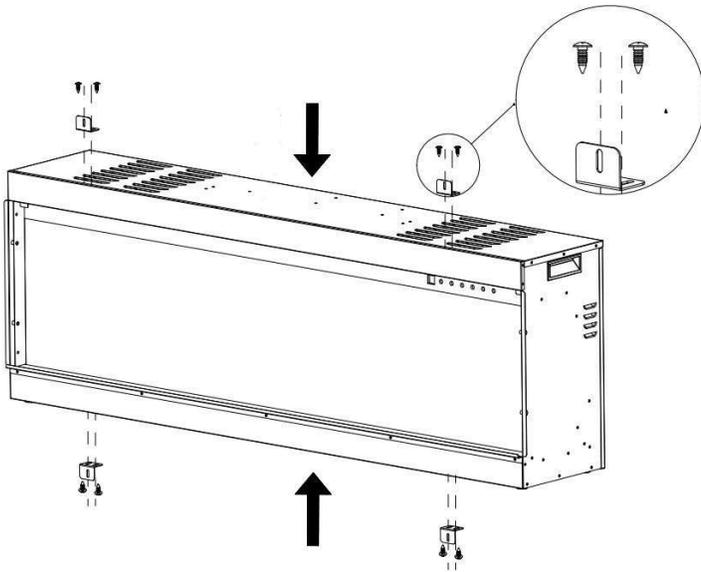
For wall installation devices: 5. Make an opening for the fireplace according to requested measurement. Insert the fireplace into the wall opening. Drive the mounting screws into the brackets and the wall studs. Plug in and check if the fireplace works properly. If so, move on to next step.
