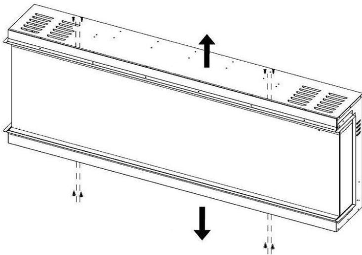
4. Fix the brackets with the screws in the previous step.
