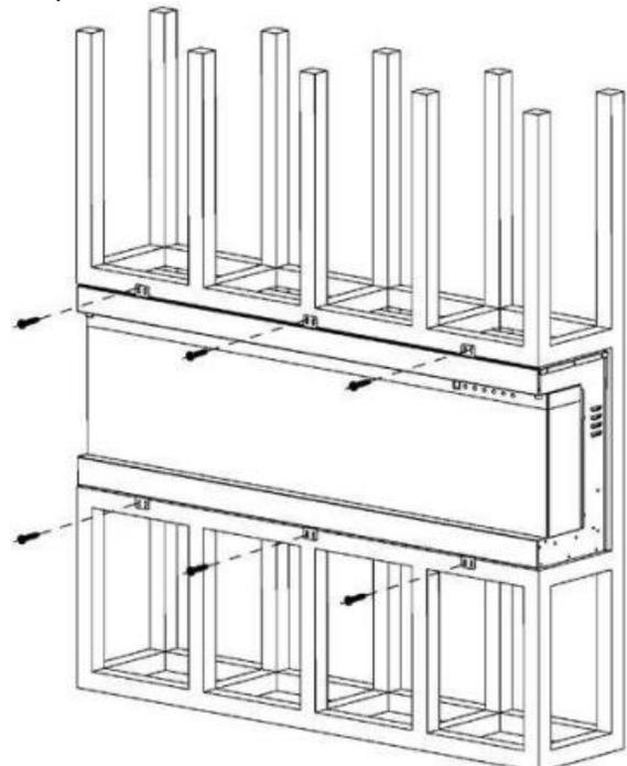
For wall installation devices: 6. Cover the glass panel with protective plastic bag and install plywood or drywall.
