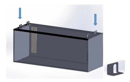
Assemble the 4 supplied mounting brackets under the housing of the Incanto. The positions have already been determined. Attention: the slots have to correspond with the notch in the housing.
