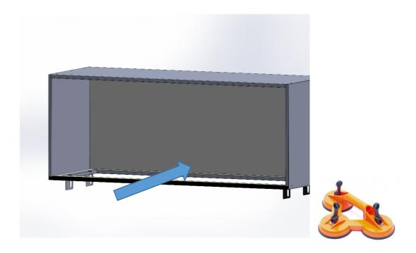
Carefully mount the glass back plate with the supplied sucking cups (orange part). Place it on the glass back plate and pull the levers when you put pressure on the glass. Attention: Convince yourself that the sucking cups have been mounted to the glass in the right way and that they have enough adhesive strength.
