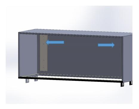
Assemble the housing against the wall at the height that you have determined. Use the supplied screws and plugs.
