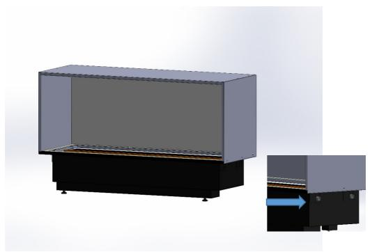
Place the Mistero unit in the housing. The round tabs on the unit exactly fit into the openings of the housing till the unit finally stick in the four mounting brackets.
